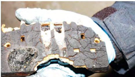
The effect of fire on a socket-outlet (Photo courtesy of Greater Manchester Fire & Rescue Service).
