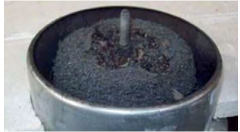
Fire rated Ceiling Air Valve sealed after a fire Photos courtesy of Tenmat Ltd.
